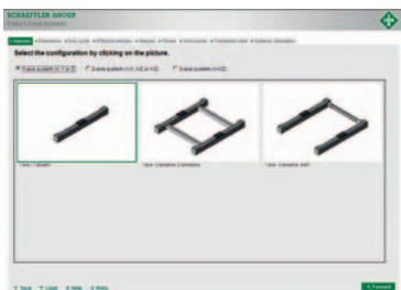
① – ③ Selection of preconfigured 1, 2, or 3-axis positioning systems
