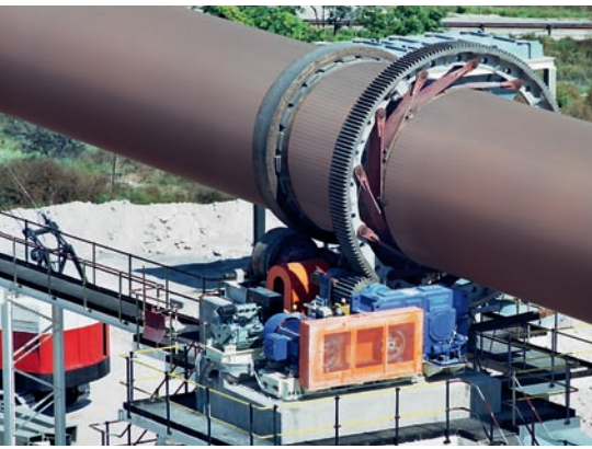
Flender gear units used as tube-mill drives – a proven area of application for the INA and FAG rolling bearings with their high load capacity (Photo: Flender)
