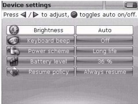
FAG Top-Laser EQUILIGN offers two display brightness modes: automatic mode and manual mode. Automatic mode automatically adjusts the brightness to the ambient lighting conditions.
