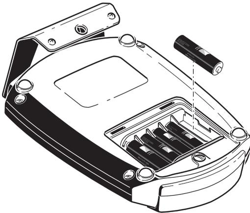
Note the battery polarity when inserting the batteries (alternating +/-).
