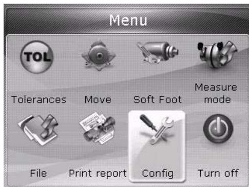
When 'Config' is highlighted, press
