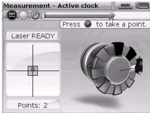
Rotate the shafts to the next measurement position and take a measurement point. Three or four measurement values (depending on the default settings; see Page 24) from the eight possible positions are required for an analysis of the results. Measurements can be carried out in any order. The results screen opens automatically after all the required measurements points have been taken.
