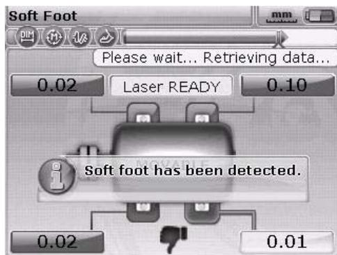
The default foot tolerance is 0.06 mm. If any single foot exceeds this tolerance, a 'thumbs down' icon appears immediately.
