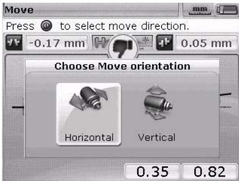
Use the [Left Arrow] [Right Arrow] keys to highlight 'Horizontal' for horizontal machine movement. Press [Enter] to confirm the selection. Live MOVE starts immediately.
