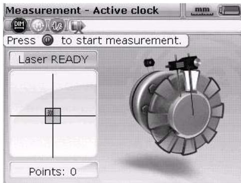
When making the adjustments mentioned above, take note of the LEDs on the FAG Top-Laser EQUILIGN computer and the laser dot on the display screen. The LED lights up in green when the laser position is suitable and measuring can commence. The LED lights up in blue when the laser beam is centred exactly in the target box.
