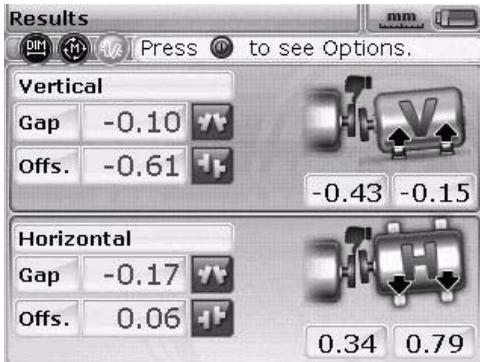
The vertical foot results show that the back feet on the right-hand machine must be raised with a 0.45 mm shim.
