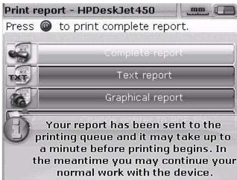
Alternatively, the measurement report can be printed directly via the results screen by pressing
