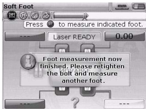
Loosen the corresponding foot anchor bolt. The measured distance by which the foot has lifted is shown on the screen.
