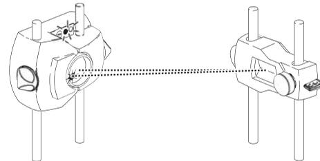
Both transducer LEDs flash alternately and the indicator LED on the FAG Top-Laser EQUILIGN computer lights up YELLOW.
