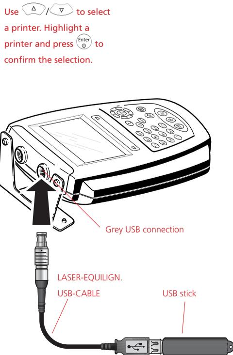
Measurement files can also be saved directly as PDF files by selecting the 'PDF file' option, which enables files to be shared immediately and printed by any printer compatible with Windows.
