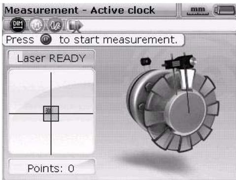
Active clock is the default measurement mode. In this mode, measurement points are taken at any three or four points in the eight possible sectors. Three measurement points are sufficient to determine the alignment status. You can find information about static measurement mode (default) in the 'Alignment options' chapter on Page 79.
