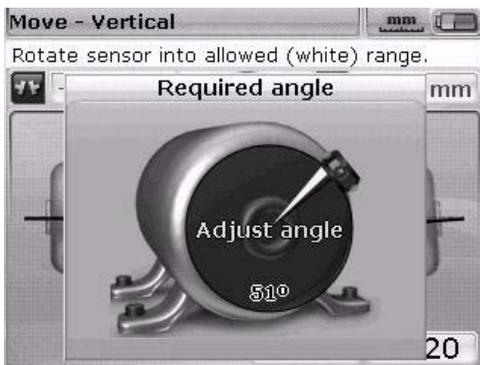
Live MOVE resumes automatically once the shaft is rotated back to its previous 45° position.
