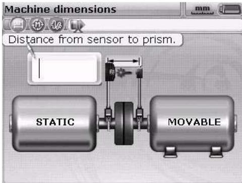
An editing box appears with information about the measurement that must be entered or edited. Any missing measurements that are required can be entered directly using the data entry keys.
