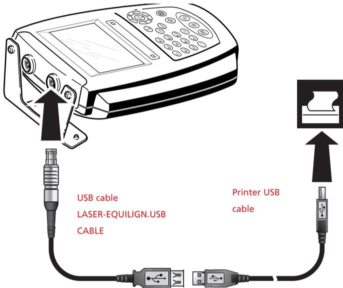
The FAG Top-Laser EQUILIGN computer is connected to the printer via the short USB cable and the printer USB cable. The printer USB cable is a printer accessory and is available from most electronics retailers.
