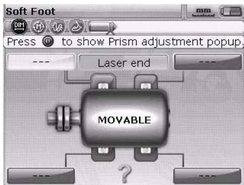
In this example, the instructions on-screen show that
