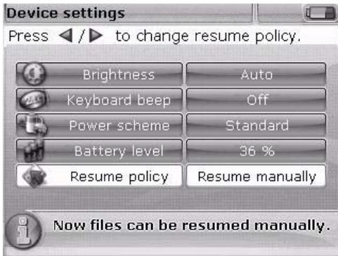
The keys can also be used to switch between the two 'Resume policy' options.
