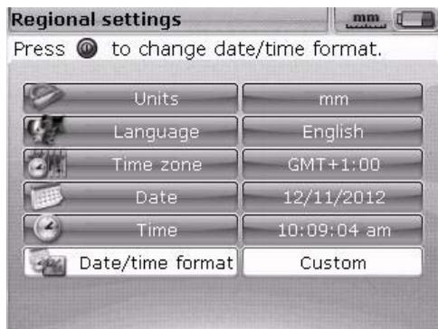
Highlight the 'Date/time format' menu item and press [Enter]. This opens a selection menu with the 'Date format' and 'Time format' menu items. Select a menu item from the pull-down menu using the [Up] / [Down] keys.
