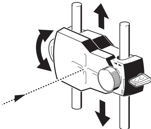
cap of the reflector. If the dust cap is on, the message 'Laser off' will appear on the screen and the indicator LED for the alignment status on the FAG Top-Laser EQUILIGN computer will light up in red.
