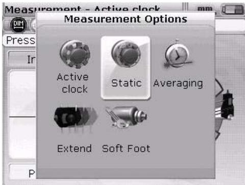
The 'Measurement Options' screen can only be accessed if all necessary machine data has been entered in the measurement file that is currently open.
