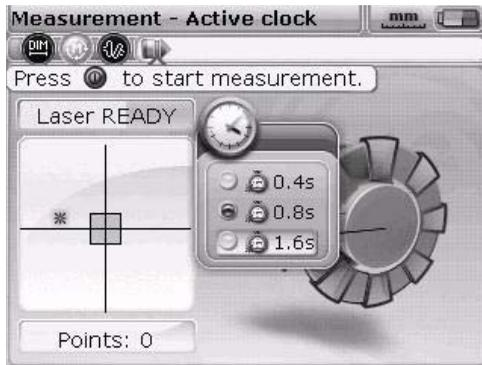
The setting options for calculating the average range from 0.4 seconds (smallest value) to 1.6 seconds (largest value).
