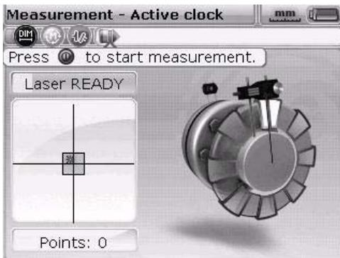
After taking the measurement, rotate the shaft into the next sector and repeat the process.
