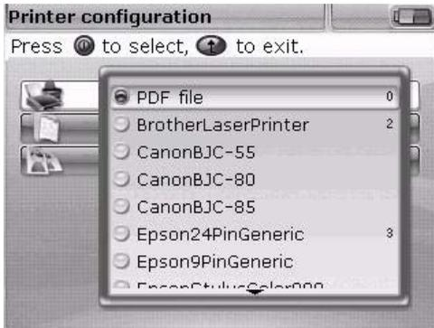
If 'PDF file' is selected, press
