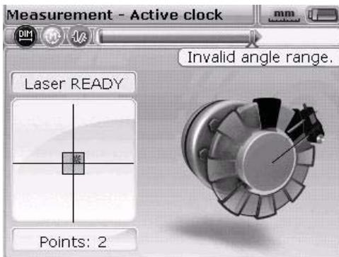
In this example, the transducer is in a sector marked in black. No measurement can be taken at this angle.
