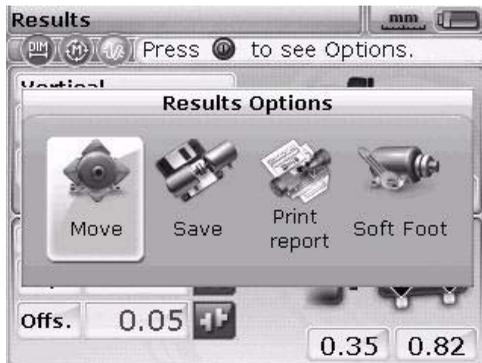
Use the navigation keys to highlight the 'Move' icon, then press
