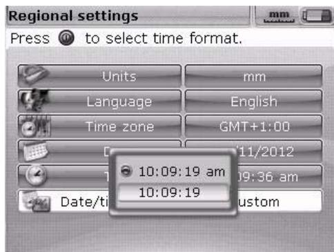
Under 'Time format', you can select whether the time is displayed in the 12-hour or 24-hour format. Confirm your selection by pressing [Enter]. Under 'Date format' you can select whether the date is displayed as dd-mm-yyyy or mm/dd/yyyy.
