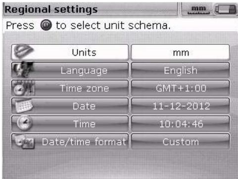
Highlight the 'Units' menu item using the keys and press to confirm the selection. The measurement units available for selection are American, English and metric units (SI units). Select the desired system of units using the keys. Press to confirm the selection.
