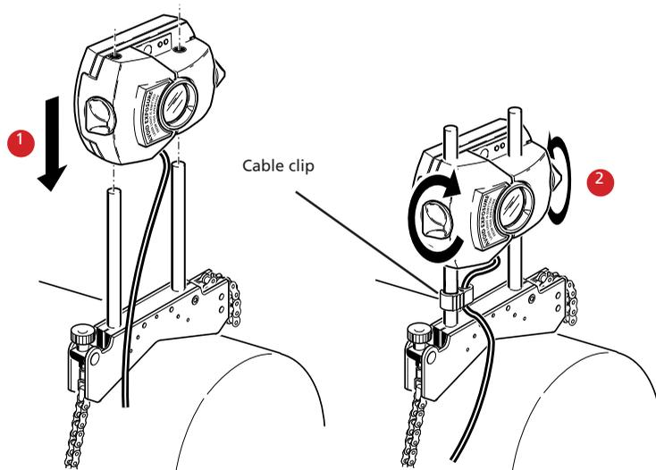
1. Loosen the yellow locking screws and slide the transducer onto the support rails.
