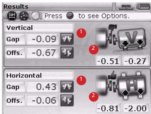
The coupling values (1) and foot values (2) are displayed in both horizontal and vertical directions.
