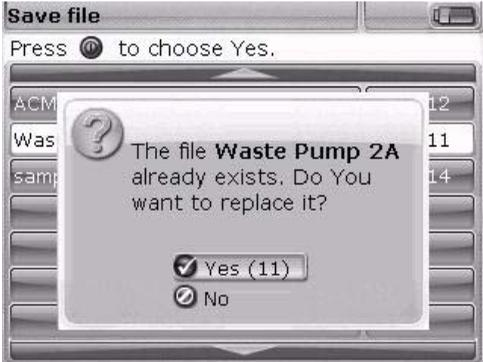
Overwriting the last version ensures that the measurement file is saved together with the latest alignment results.
