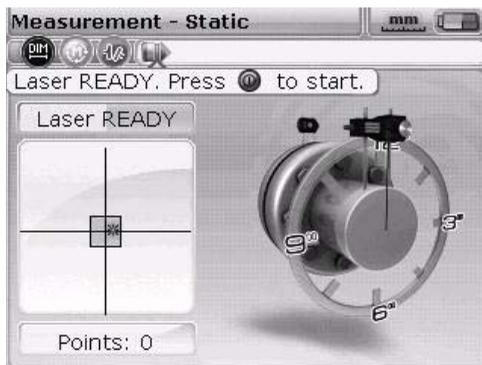
Move the clock hour hand to the next 45° position by pressing the navigation keys.
