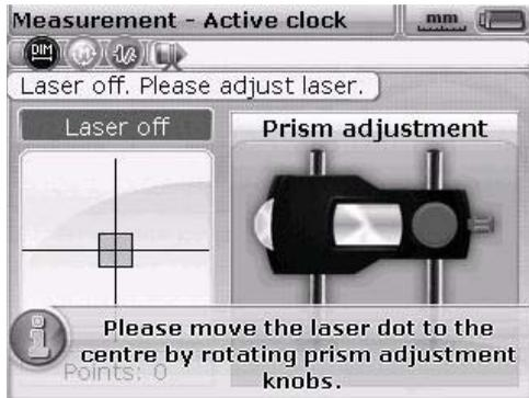
The transducer and the reflector must be arranged so that the laser beam strikes the reflector and is reflected back into the transducer.
