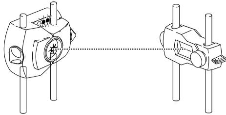
Both transducer LEDs flash slowly in unison and the indicator LED on the FAG Top-Laser EQUILIGN computer lights up GREEN.
