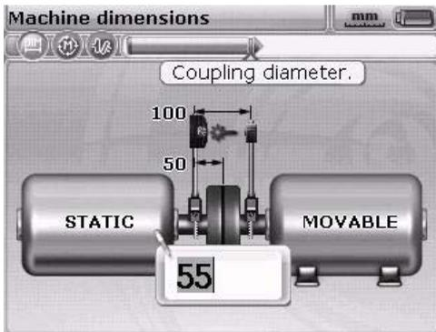
Alternatively, auto flow mode can be overridden using the **⏪** key. This allows activation of advanced entry mode, which can be used to access editing boxes and machine elements using the navigation keys.
