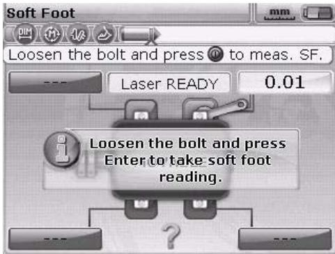
Loosen the corresponding foot anchor bolt then press the
