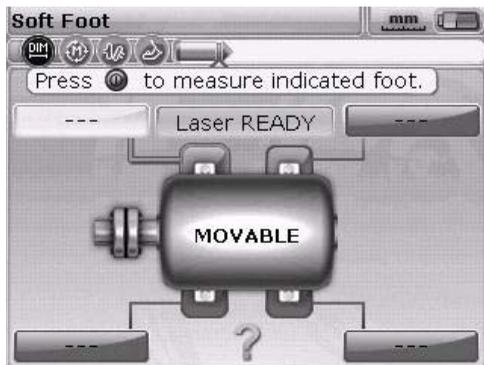
Centre the laser beam and press the
