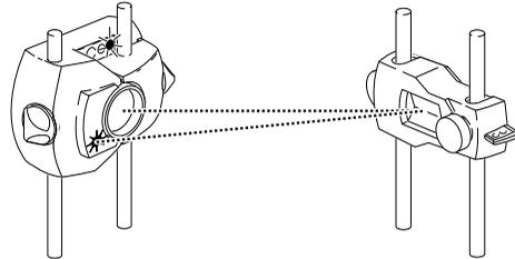
The RED LED on the transducer flashes quickly, the GREEN LED is off and the indicator LED on the FAG Top-Laser EQUILIGN computer lights up RED.
