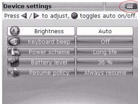
The charge level of the battery is displayed in the top right-hand corner of every screen.
