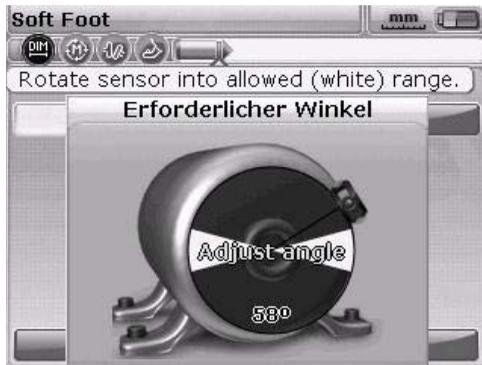
Rotate the shaft to the correct 3 o'clock or 9 o'clock position (green segments in the circle) and continue the measurement process.
