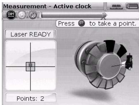
If, in active clock mode, the number of measurement points has been set to four, the results can be accessed after three measurement points have been taken by pressing .
