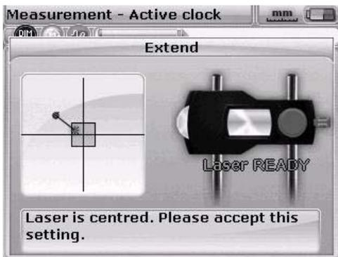
5. Once you have centred the laser point, the LED on the computer lights up blue. The set laser beam position is recorded and automatically becomes the end point for laser beam deviation.
