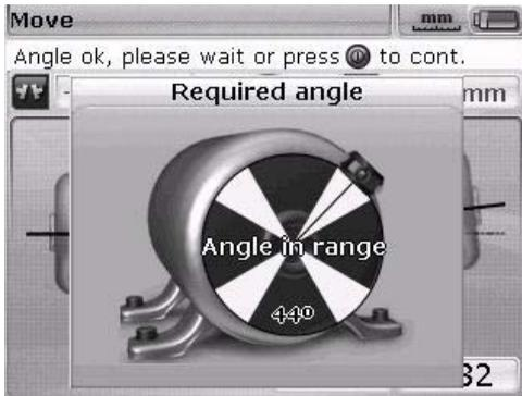
If the laser is centred and the shaft is rotated into one of the green sectors, then the screen to select the direction of movement will open automatically.
