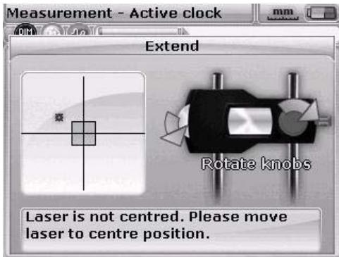
4. Re-adjust the laser beam to strike the target box using the yellow adjustment knob and the thumbwheel on the side of the reflector.
