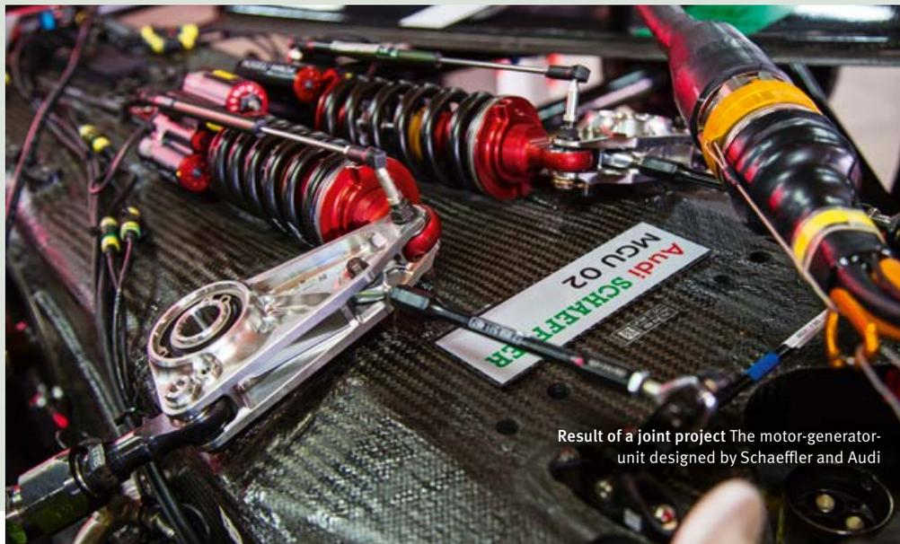
Result of a joint project The motor-generator unit designed by Schaeffler and Audi
